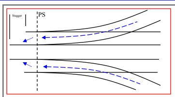
The stagger of the joints ahead of the switch point should be as shown above, in my opinion. The small arrow represents the driving force of the lead wheel before it straightens out.
